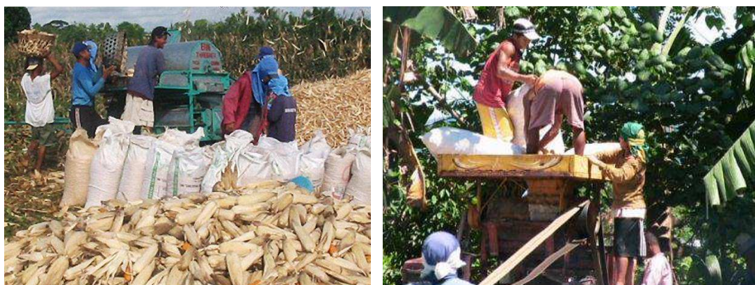
Picture 3-10. Corn shelling with 2 kinds of shellers: hopper at the side and on top
