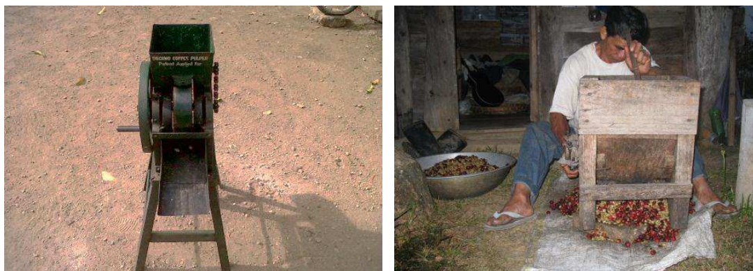
Picture 3-11. Mechanical and wooden depulpers used in wet processing of coffee
